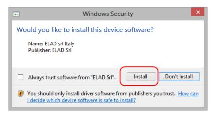
Let the hardware installation automatically completes and, at the procedure ending, click on "Close"; then disconnect and connect FDM-S2 device on the same USB socket.
